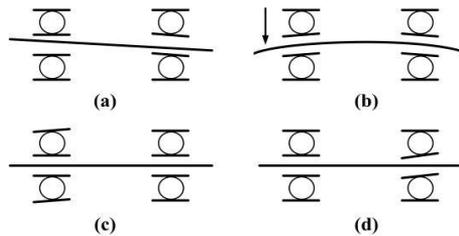
**Fig. 4** – Misalignment of bearing installation: (a) Misalignment; (b) Shaft deflect; (c) Outer race damage; (d) Inner race damage
