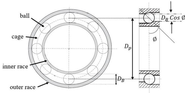
**Fig. 3** – Induction motor bearing construction.
