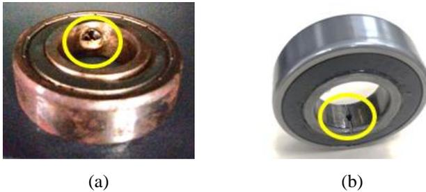
**Fig. 5** – Bearing fault conditioning: (a) Fault#1; (b) Fault#2.
