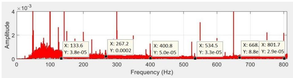
**Fig. 7** – Healthy motor sound frequency at no load.
