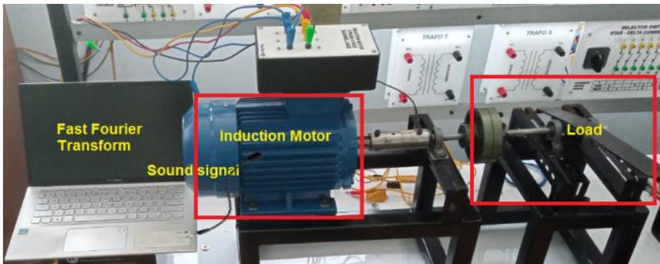
**Fig. 2** – Implementation of the fault detection system.
