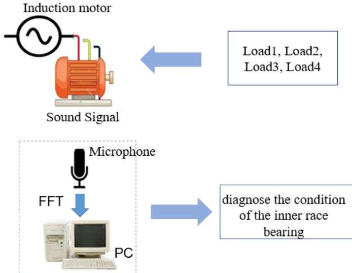
**Fig. 1** – Block diagram of fault detection configuration on inner race.
