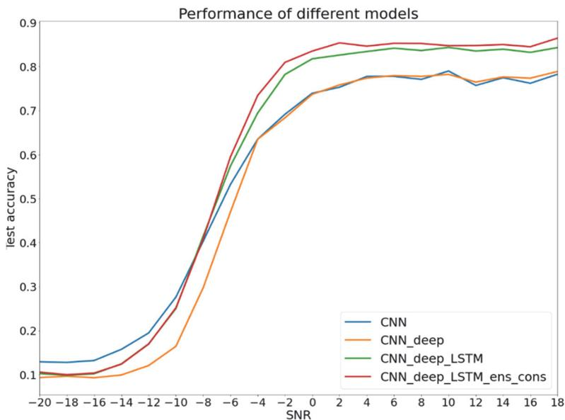
Fig. 13 – Performance comparison of different deep learning models with respect to different SNRs.
