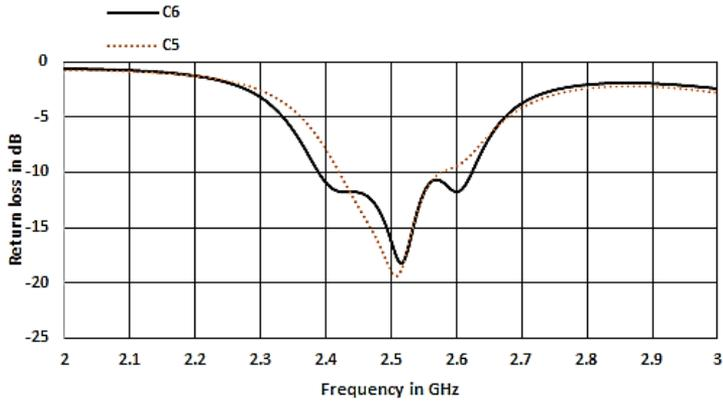
**Fig. 9** – Return loss variation for configurations C5 and C6.
