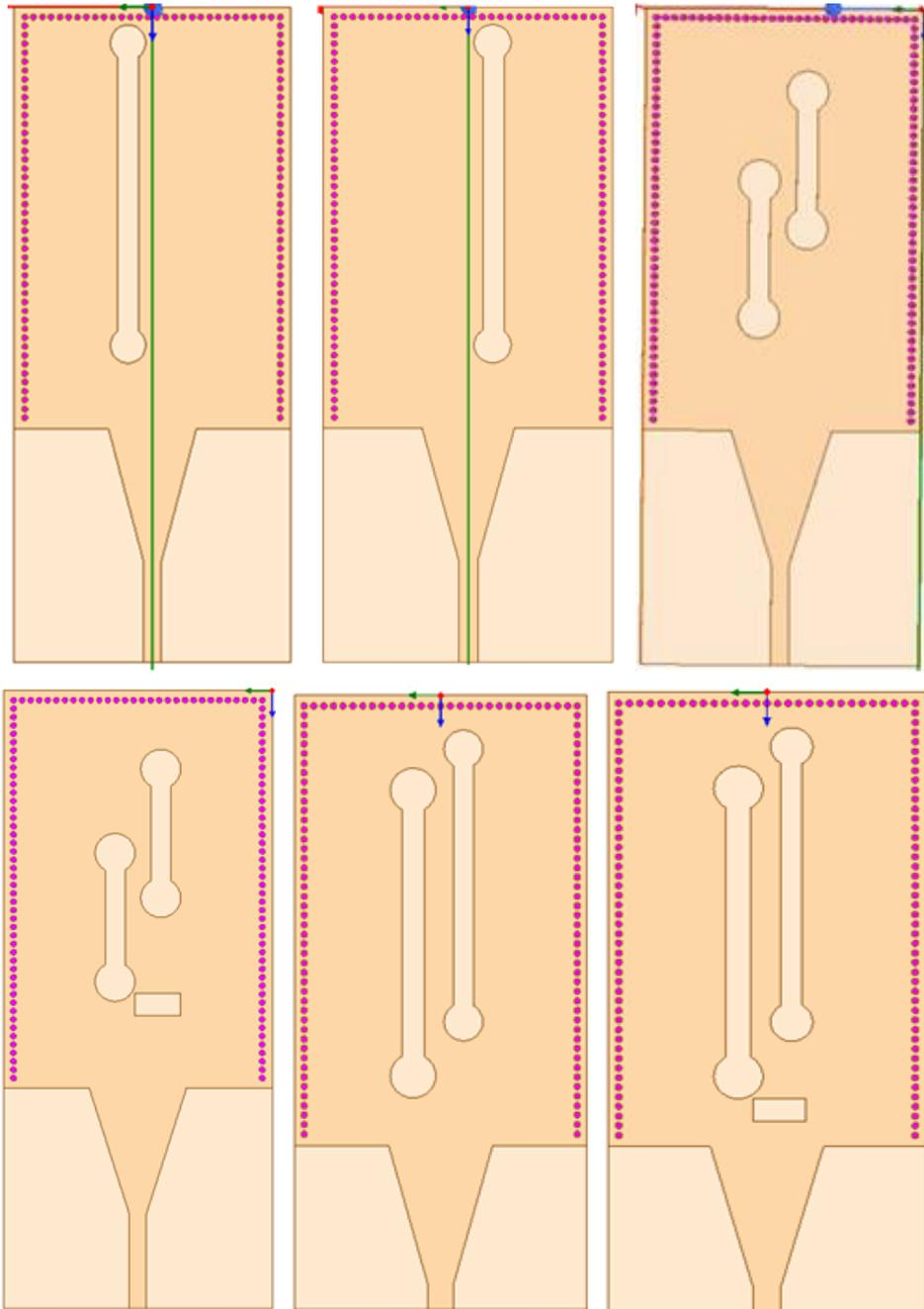
**Fig. 3** – Configurations (C1~C6) of the SIW antenna.
