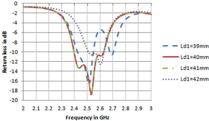
**Fig. 7** – Return loss variation when width  $L_{d1}$  is changed.
