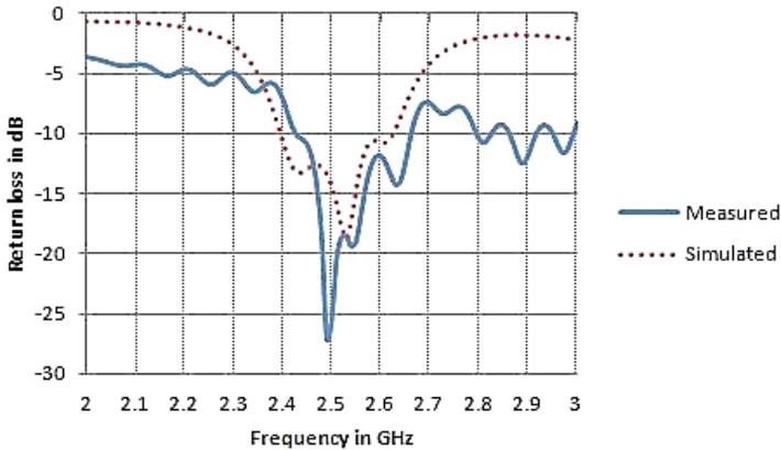
Fig. 13 – Comparison between the simulated and measured return loss of the proposed antenna.
