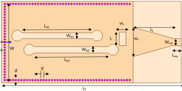
Fig. 2 – Proposed antenna: Top view.
