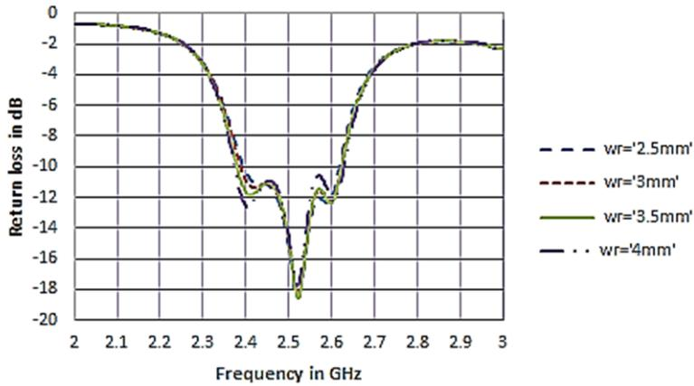
**Fig. 10** – Return loss variation when width  $w_r$  is changed.
