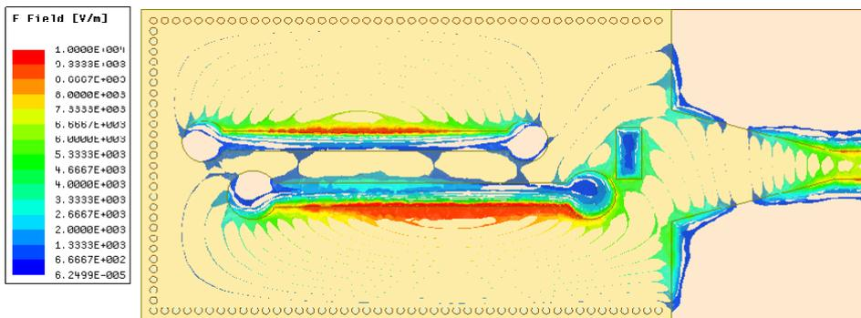
**Fig. 4** – Electric field distribution.
