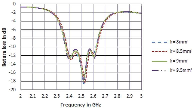
**Fig. 11** – Return loss variation when width  $l_r$  is changed.
