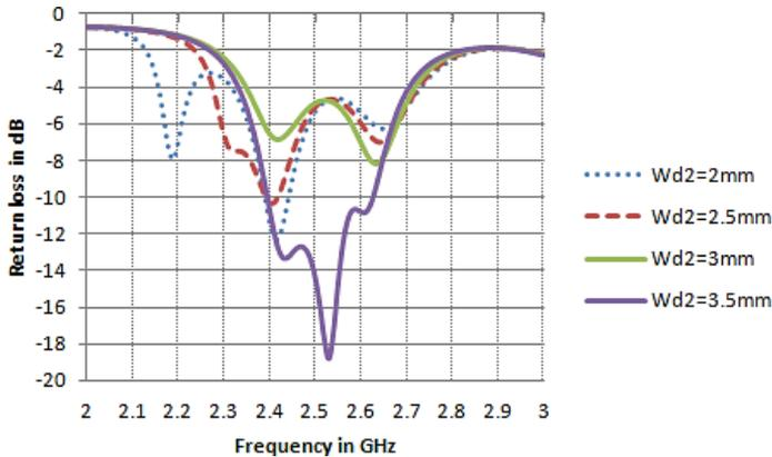
**Fig. 6** – Return loss variation when width  $W_{d2}$  is changed.
