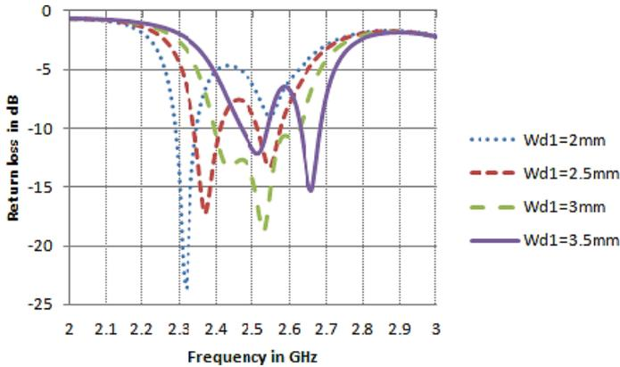
**Fig. 5** – Return loss variation when width  $W_{d1}$  is changed.
