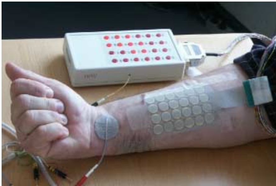
Fig. 3 - The application of the Actitriode® in experiments. The round Pals Platinum electrode ( D = 3.2cm ) was used as the anode over the carpal tunnel, and the Actitriode® (cathodes) were positioned on the dorsal and volar sides of the forearm.
