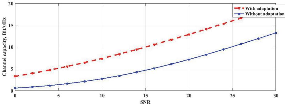
**Fig. 9 – The capacity of the data channel depending on the specified SNR.**
