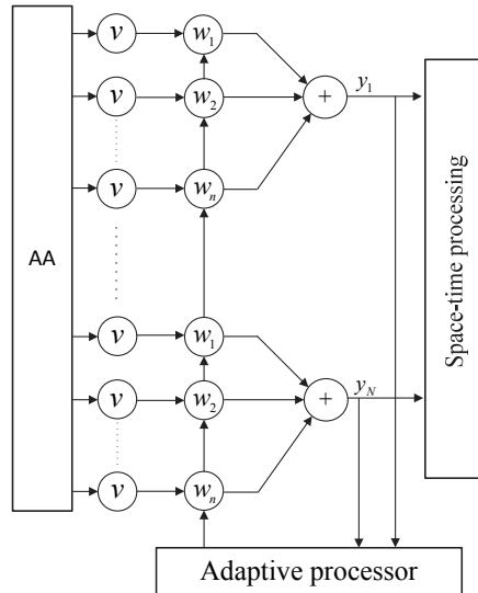
**Fig. 4 – Block diagram of the receiving antenna system and adaptation unit.**
