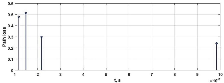
**Fig. 1 – Pulse characteristic of 3GPP data transmission channel.**
