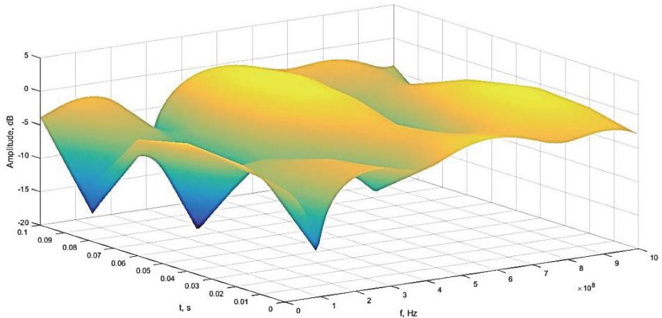
**Fig. 2 – Frequency response of 3GPP data transmission channel.**
