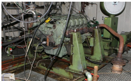
Fig. 2 – OM403 engine on test stand.
