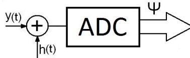
Fig. 2 – Block diagram of application of a uniform random dither h to the measured signal y .
