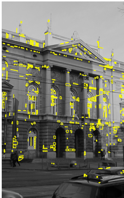
Fig. 9 – Detected MSER features in the example image.
