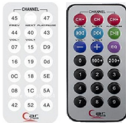
Fig. 1 – Remote control device with defined button codes (left) and image of remote control (right).
