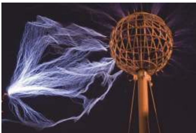
Fig. 7 – The discharges with the length of over 3m at the top of TT during the ignition of the University torch at the opening ceremony of the 25th Summer Universiade 2009 in Belgrade.
