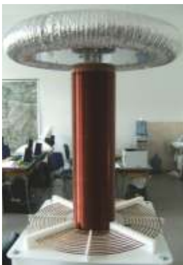
Fig. 3 – The TT manufactured at the School of Electrical Engineering in Belgrade in 2006. Output voltage is around 700 kV, working frequency is 100.5 kHz, power 2.5 kVA.
