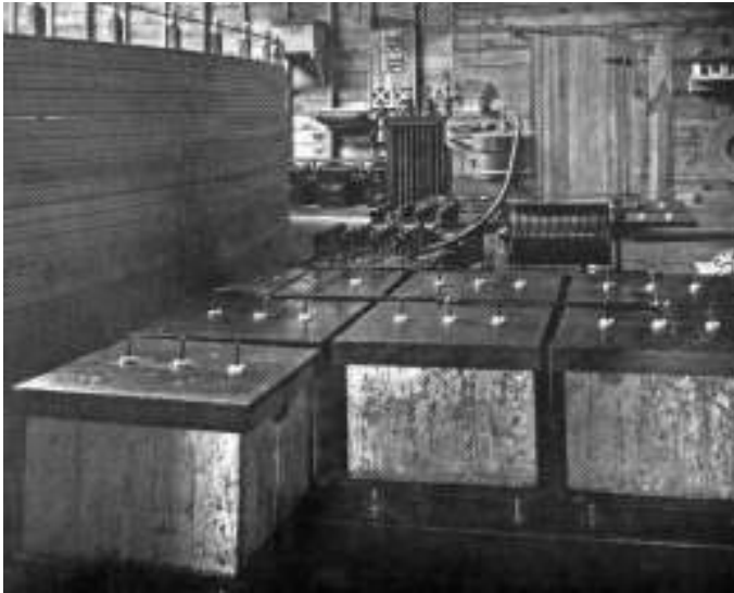
Fig. 11 – The bank of capacitors for the primary circuit for high frequency transformers in Colorado Springs in 1899. In the background, one can see the variable inductance coil. (Source: Popovic, Vojin, Nikola Tesla - From Colorado Springs to Long Island, Belgrade, Nikola Tesla Museum, 2008, p.302).
