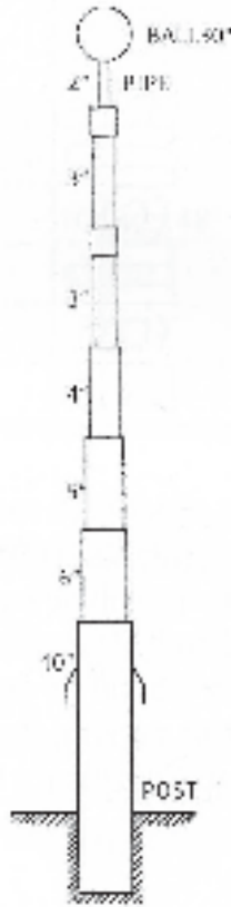
Fig. 12 – The construction and the dimensions (the diameters are given in inches) of steel antenna in experiments in Colorado Springs, the lower part of the pole (antenna carrier) is the wooden beam (Source: Popovic Vojin, Nikola Tesla – From Colorado Springs to Long Island. Belgrade: The Nikola Tesla Museum, 2008, p.187).
