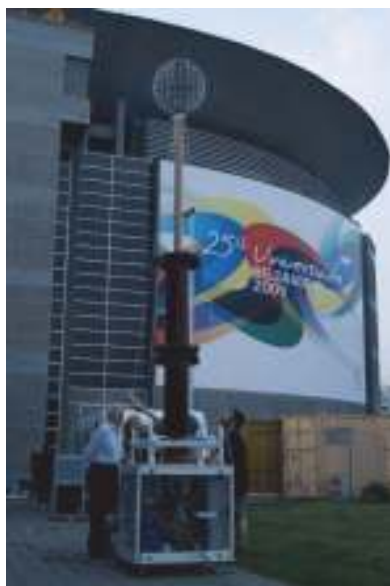
Fig. 6 – The TT made at the School of Electrical Engineering in Belgrade for the purpose of the opening ceremony of the 25th Summer Universiade 2009. Project leader Prof. Jovan Cvetić. Installation is attended by academician Prof. A. Marinčić, SANU gallery curator B. Božić and BSc. V.Malić. The total height of TT is 6m, while the length of the secondary coil is about 2m. The output voltage of 1.5 MV, the operating frequency is 52 kHz at input power of 10 kVA.
