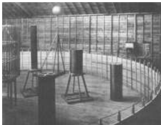
Fig. 9 – The interior of the laboratory in Colorado Springs in 1899. The part the high-frequency transformer with a diameter of 15 m (wound on the outside of the wooden fence) as well as the large extra coil (the far left) with several smaller ones can be seen. (Source: Popovic, Vojin, Nikola Tesla - From Colorado Springs to Long Island, Belgrade, Nikola Tesla Museum, 2008, p.302).
