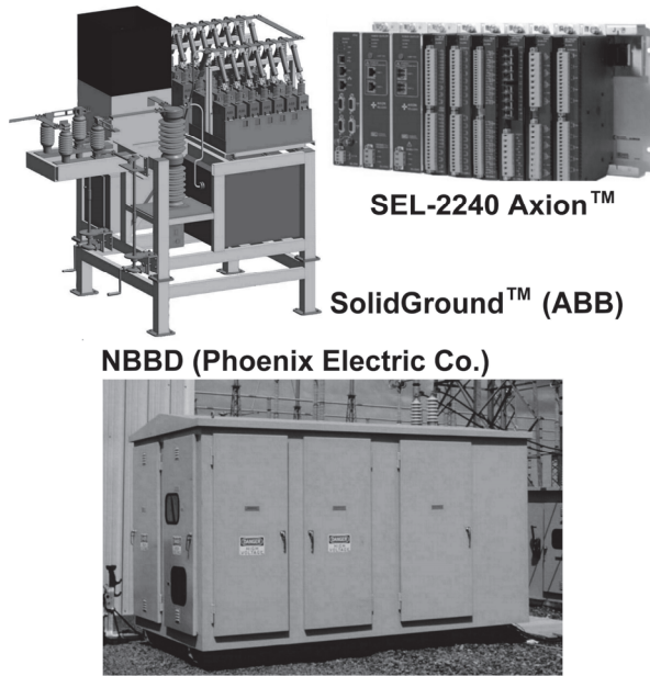
Fig. 7 – GIC blocking unit integrated into the power transformer neutral conductor. Above is the unit manufactured by ABB Company equipped with controller manufactured by SEL, below is the unit designed by Phoenix Electric
