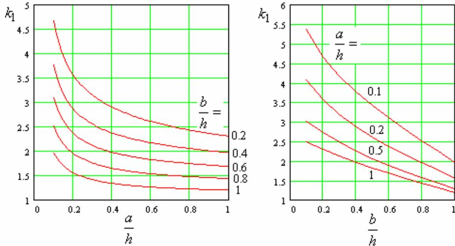
**Fig. 3** - Coefficient  $k_1$  from formula (8), calculated with (24).
