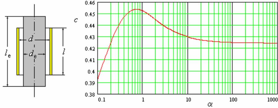
**Fig. 1** - Coefficient  $c$  for equivalent gap.
