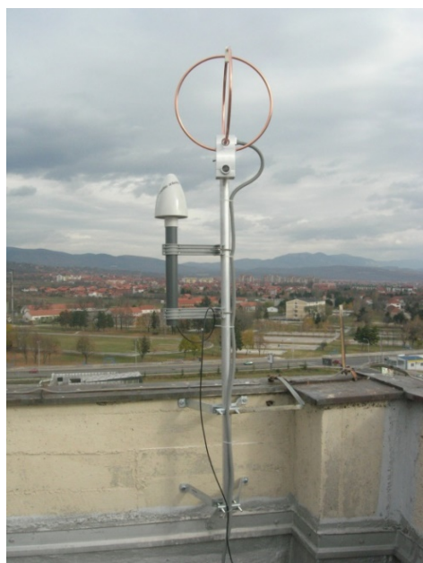
Fig. 4 – Cross-loop and GPS antenna in Niš.
