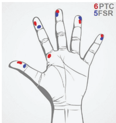
Fig. 6 – The map of optimal sensors can be constructed using only six PTC thermistors and five FSR sensors.
