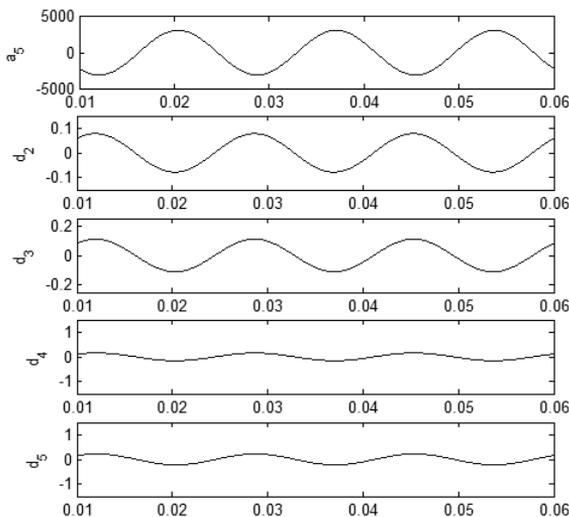
**Fig. 5** – The resulted approximations and details in different levels obtained for the voltage signal of line AB on the condition of the single line to ground short circuit fault.
