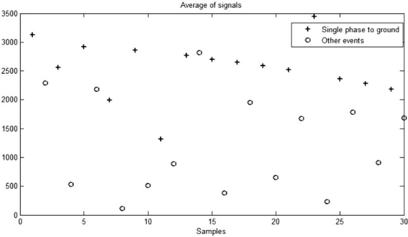
**Fig. 9** – A comparison between the values of the area under the curve of the (fifth level detail of) voltage signal during the single-phase fault occurrence as well as the other phenomena in 30 samples of shipboard power system.
