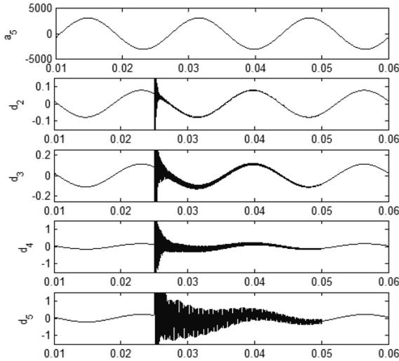
**Fig. 7** – The resulted approximations and details in different levels obtained for the voltage signal of line CA on the condition of the single line to ground short circuit fault.
