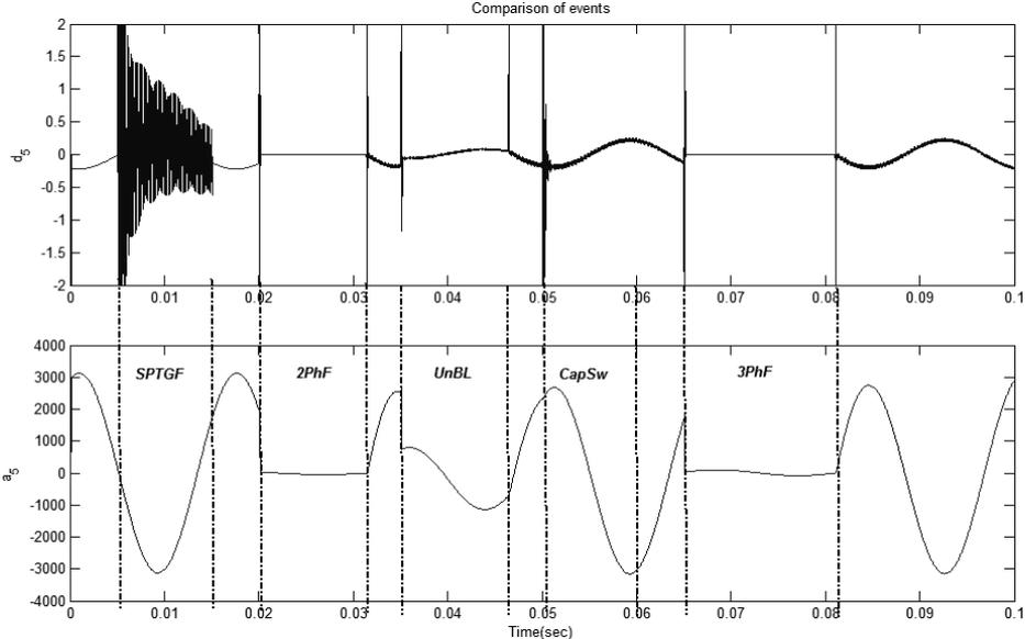
**Fig. 8** – Fifth level approximation and detail of the single line to ground fault and the other phenomena in a sample network (SPTGF: Single line to ground fault, 2PhF: Double line fault, UnBL: Unsymmetrical load switching, CapSw: Capacitor bank switching, 3PhF: Symmetrical three-phase fault).
