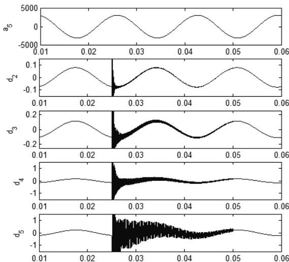
**Fig. 6** – The resulted approximations and details in different levels obtained for the voltage signal of line BC on the condition of the single line to ground short circuit fault.
