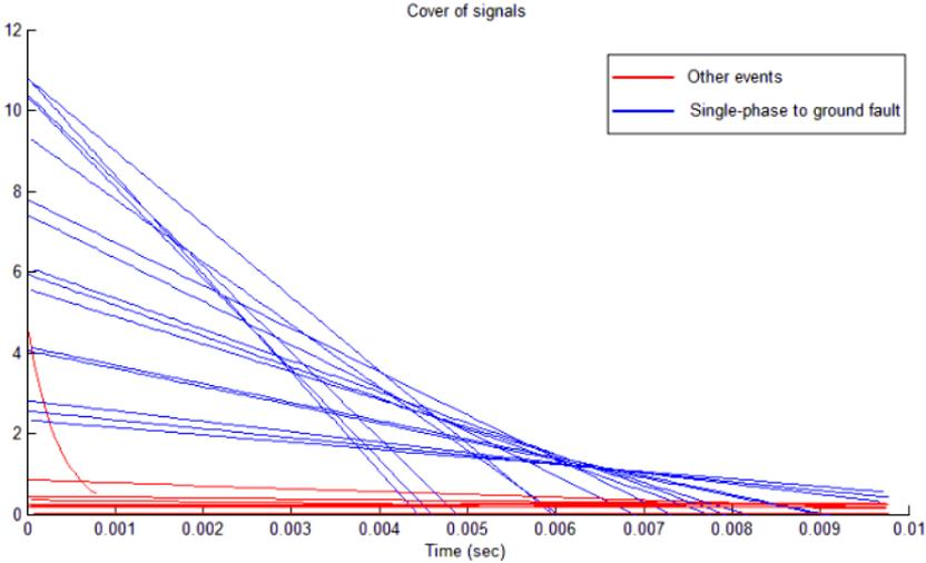
**Fig. 10** – A comparison between the curve sheath for the single phase to ground fault and the other phenomena in 30 different samples of shipboard power system.
