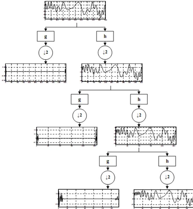
Fig. 1 – Schematic manner of Multi Clarity Decomposition for a signal.
