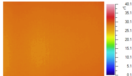
Fig. 5 – Outer surface of the wal (thermovision image).
