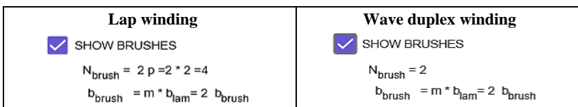
Fig. 18 – Calculation of brushes number and their width.
