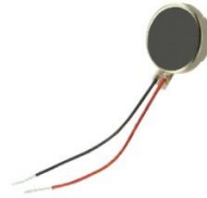
Fig. 12 – Motor for vibration stimulation.
