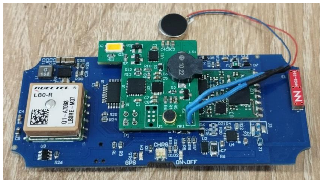
Fig. 16 – Printed circuit board of the Canandi collar system with the upgraded circuit board of designed system.
