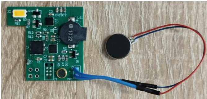
Fig. 15 – Assembled printed circuit board.
