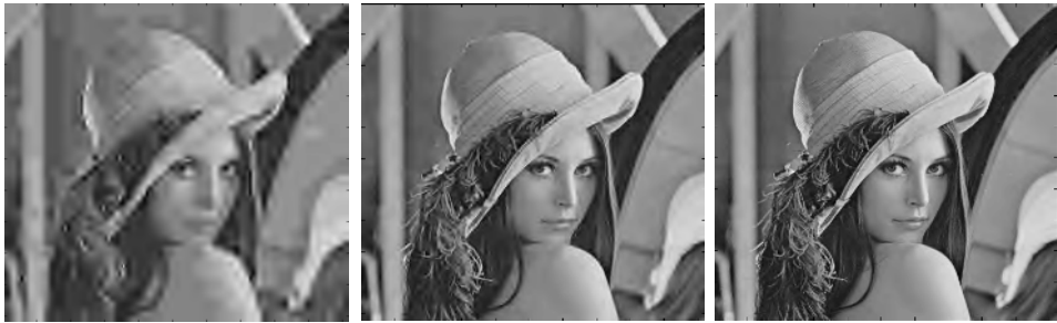
(a) Ratio = 98.44 % ; PSNR = 24.50dB MSSIM = 0.68
