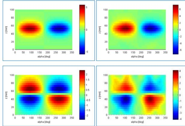
Fig. 7 - Distribution of magnetic flux density,  $B_r$  (up) and  $B_z$  (down) components calculated by analytical (left) and FEM (right) methods.
