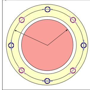
**Fig. 10** - Ring with 8 2D sensors ( $B_r$  &  $B_z$  components).
