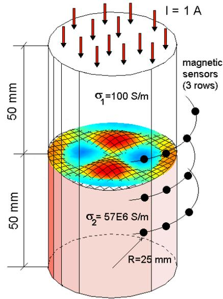
**Fig. 2** - *Highly simplified aluminum reduction cell model – cylinder with two conducting fluids.*
