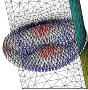
**Fig. 4** - Current density distribution near the interface.
