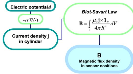
Fig. 5 - Flowchart of forward calculations using analytical method.
