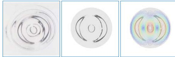
**Fig. 12 -** Photo snapshot of the interface surface (experiment) compared with the curvature distribution of  $\eta_{12}$  mode.
