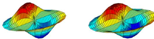
**Fig. 13 -** Original  $\eta_{12}$  mode (left) and the interface shape (right) reconstructed from the noisy  $B_r$  &  $B_z$  distribution.
