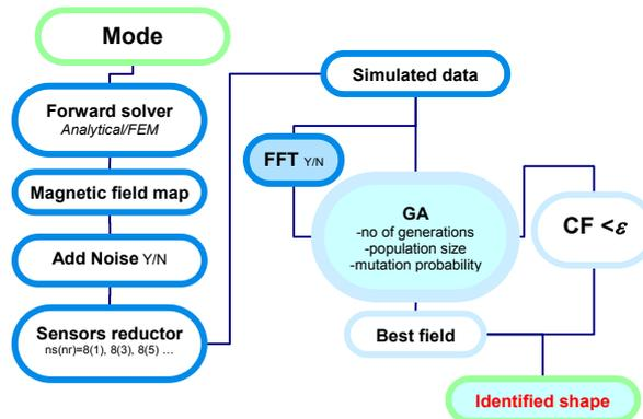
Fig. 8 - Flowchart of the interface shape reconstruction.
