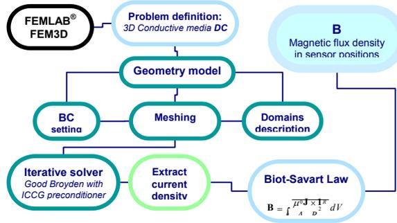
Fig. 6 - Flowchart of forward calculations using finite element method.
