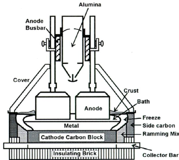
Fig. 1 - Scheme of an aluminum reduction cell.
