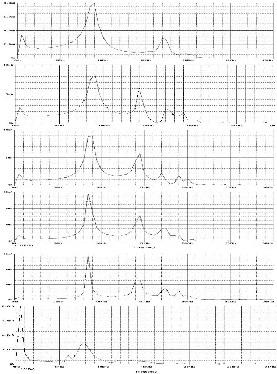
Fig. 5 – FFT of the PD signal captured at bushing tap for various PD source locations for analytically simulated parameters.
