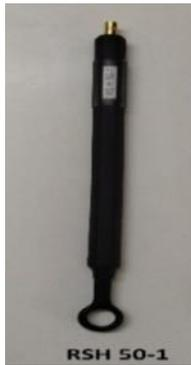
**Fig. 10** – Near magnetic field probe RSH-50-1 type: Rohde Schwarz.
