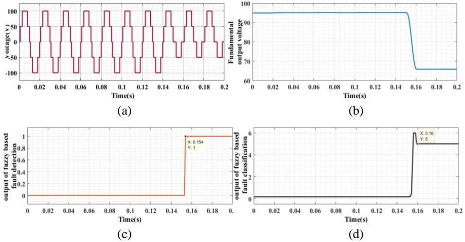
**Fig. 11** – Test findings of the class V fault: (a) Output voltage; (b) Fourier output voltage; (c) Fault diagnosis based on fuzzy logic; (d) Classification of faults based on fuzzy logic.
