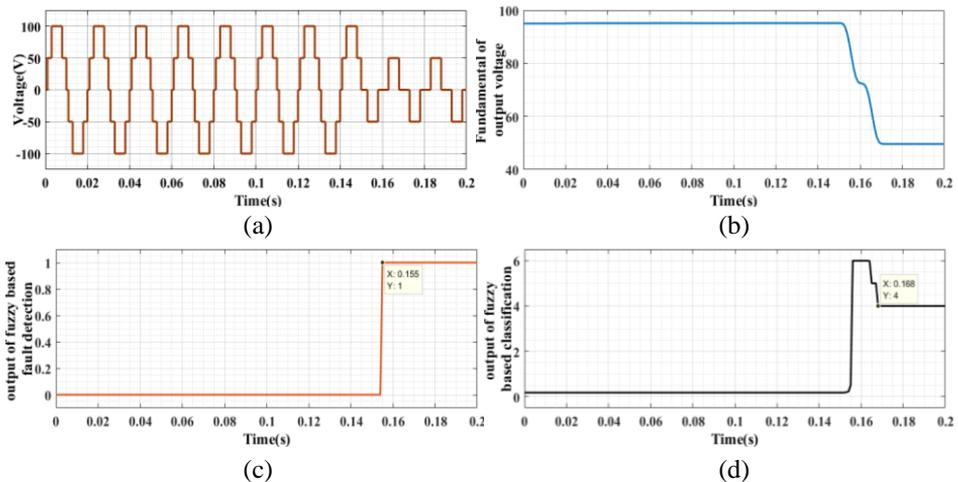
**Fig. 10** – Test findings of the class IV fault: (a) Output AC voltage; (b) Fourier voltage magnitude; (c) Fault diagnosis based on fuzzy logic; (d) Classification of faults based on fuzzy logic.
