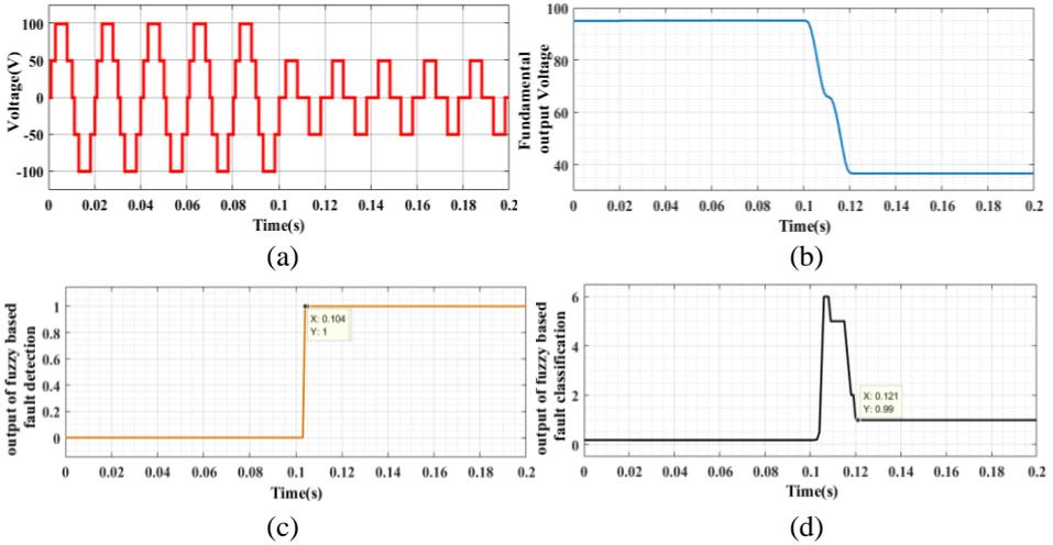
**Fig. 7** – Test findings of the class I fault: (a) Output voltage; (b) Fourier output voltage; (c) Fault diagnosis based on fuzzy logic; (d) Classification of faults based on fuzzy logic.
