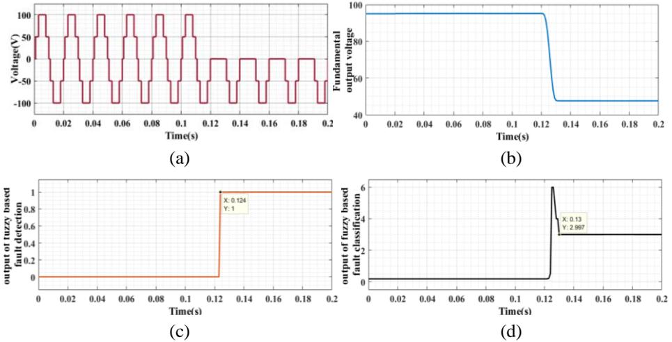
**Fig. 8** – Test findings of the class III fault: (a) Output AC voltage; (b) Fourier voltage magnitude; (c) Fault diagnosis based on fuzzy logic; (d) Classification of faults based on fuzzy logic.
