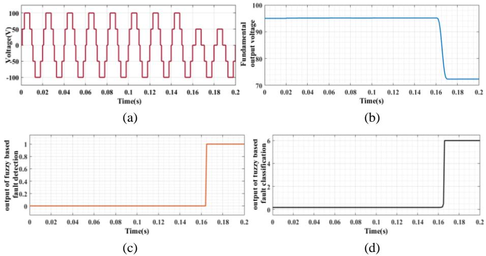
**Fig. 12** – Test findings of the class VI fault: (a) Output voltage; (b) Fourier output voltage; (c) Fault diagnosis based on fuzzy logic; (d) Classification of faults based on fuzzy logic.
