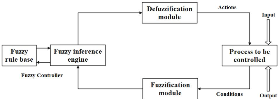
Fig. 4 – Fundamental features of a fuzzy logic control system.
