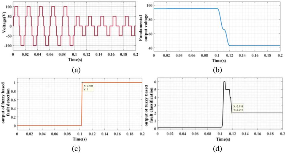
**Fig. 8** – Test findings of the class II fault: (a) Output voltage; (b) Fourier output voltage; (c) Fault diagnosis based on fuzzy logic; (d) Classification of faults based on fuzzy logic.
