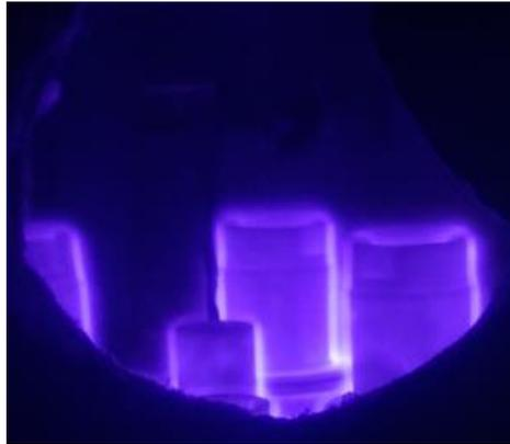
**Fig. 13** – *Glow discharge with operation of the power electronic switch.*
